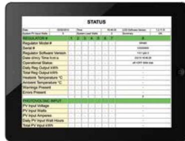
Monitor your system operation from anywhere using the Internet, or directly using a laptop, or PC. Regulator performance is updated at 15 second intervals thus providing up to date performance data. Data can be down-loaded on a daily, weekly, monthly, annual, or lifetime basis directly into MS Excel for easy graphical monitoring
