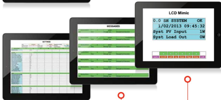
The Imark Site Explorer enables setting changes (password protected) to be done instantly. The Settings screen displays the settings for up to eight regulators in columns enabling easy settings comparisons or changes.
